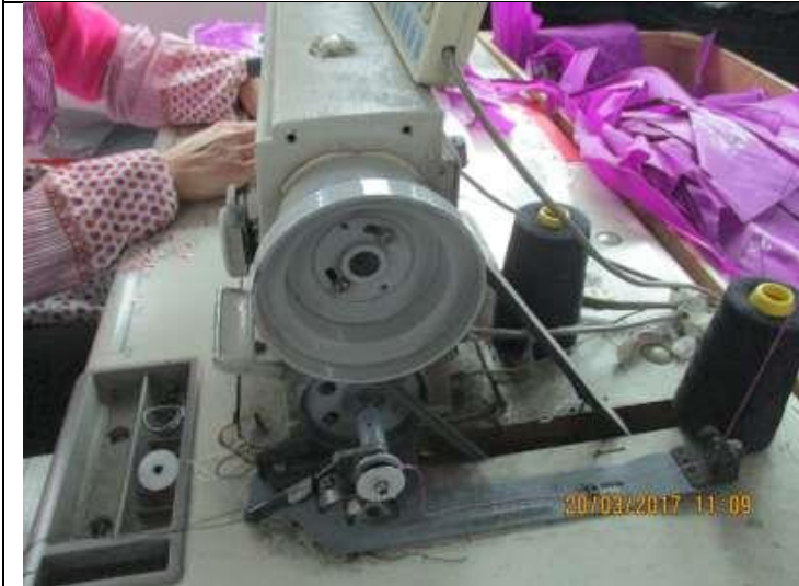
No safeguard for the belt of sewing machine
