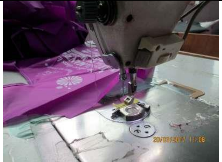
No safeguard for the needle of sewing machine
